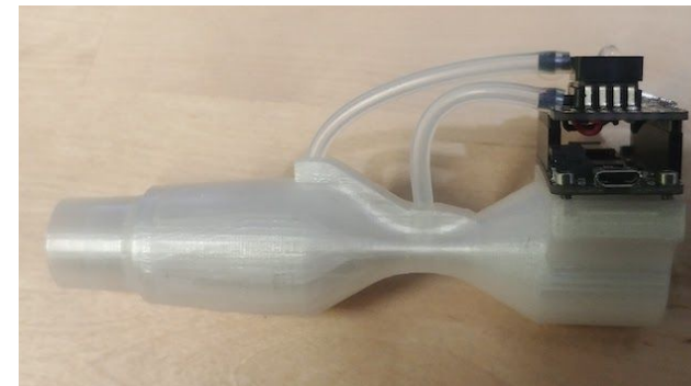
Spirotroller Game controller measuring the expiratory flow, 3d-printed, Bluetooth and USB, one button
