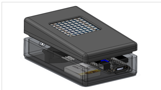
Led box Controller measuring the expiratory pressure, 3d-printed, Bluetooth and USB, 8x8 LED matrix
