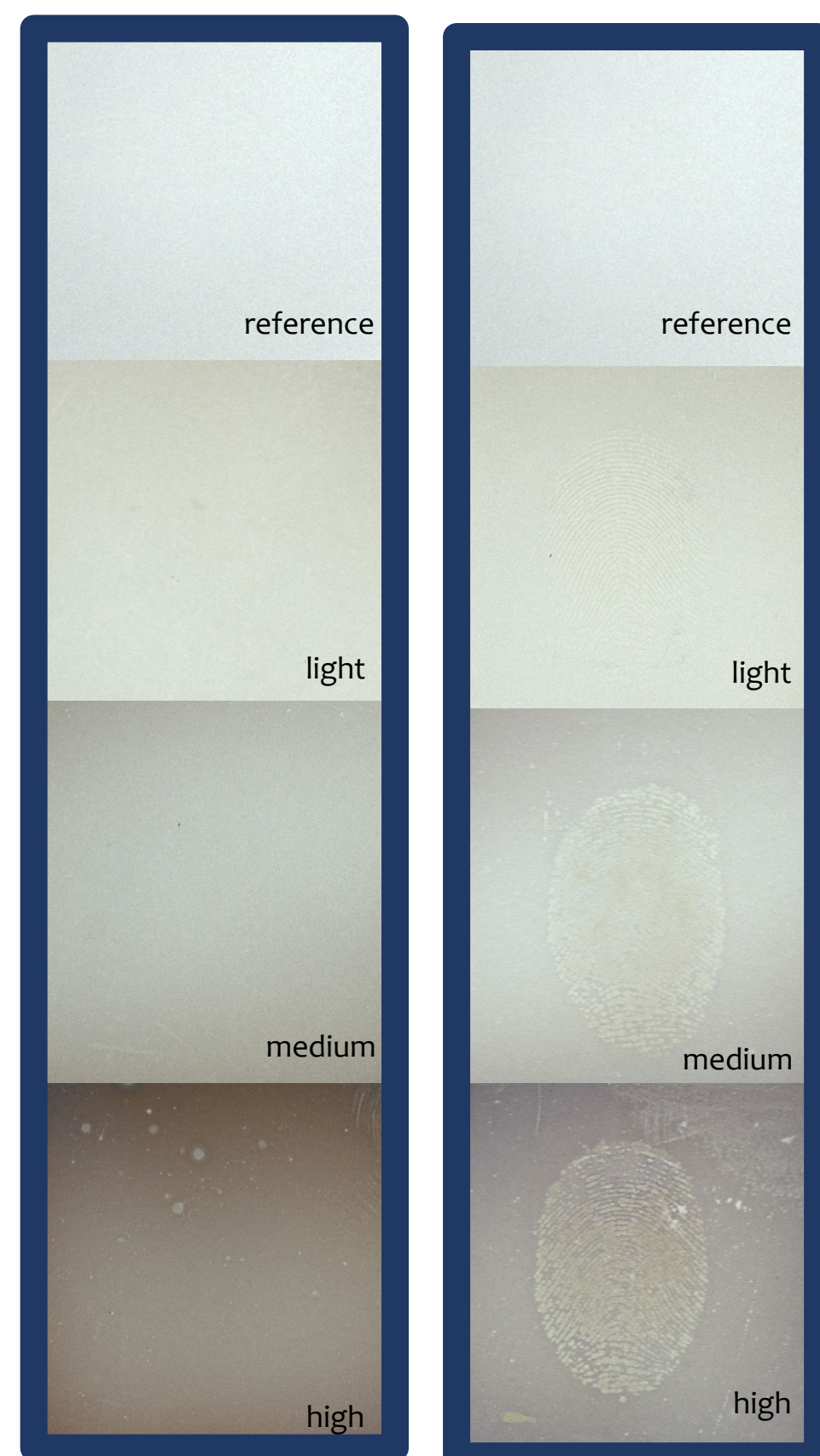
Pure Silver coupons with different degrees of tarnish (left) and placement of fingerprints (right)
