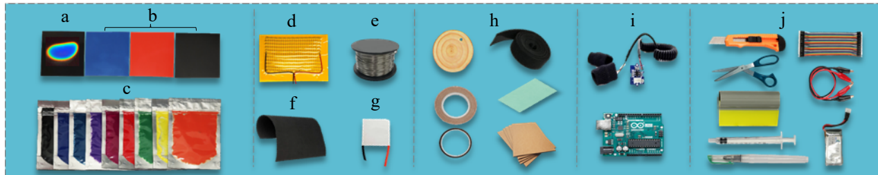
Figure 1: ThermoPixels components: a) liquid crystal sheet b) rub-and-reveal sheets c) thermochromic paints d) heating pad e) nichrome wire f) conductive fabric g) Peltier element h) insulation materials i) GSR sensor and Arduino and j) support tools
