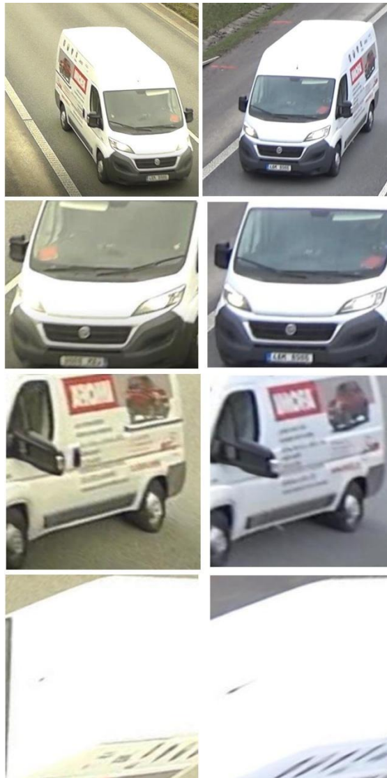
FIGURE 13: Images of a vehicle captured from different camera views, with their three sides split according to 3D bounding boxes. After performing scale-normalization on each corresponding side, differences in the appearance of image pairs can be minimized.
