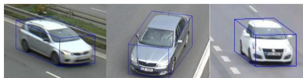
FIGURE 11: Examples of 3D bounding box construction
