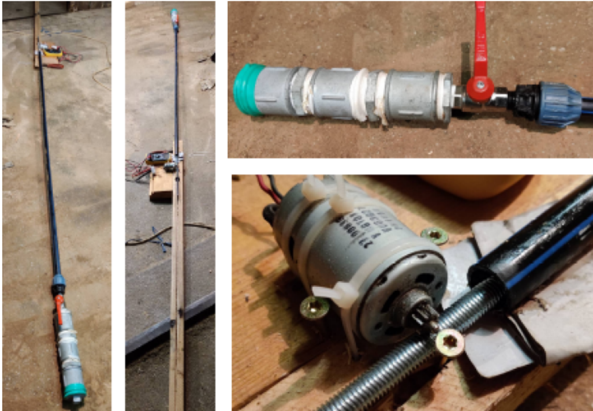
Figure 2: Experimental setup. Left and centre: expansion tube. Top right: container with valve. Bottom right: electric generator and pinion
