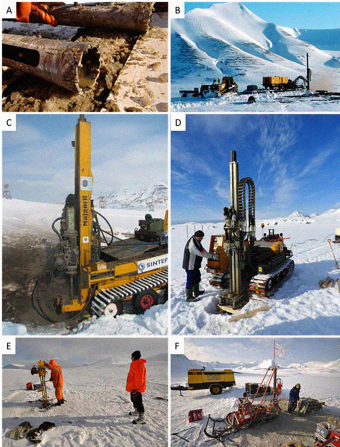
Figure 3: A) Single core barrel. Squared tungsten carbide inserts form the crown of the drill bit. (Photo: Ullrich Neumann), B) Borehole being drilled in Janssonhaugen. Drill rig, air compressor and accessories are placed onto one large sledge (Photo: Johan Ludvig Sollid). C) Rotary percussion drilling at Endalen borehole with the Geotech 504 geotechnical drill rig. (Photo: Håvard Juliussen). D) The Hornsund GM 50 GT Combi drill rig. (Photo: Tomasz Wawrzyniak). E) Russian drill rig in operation near Barentsburg. (Photo: Ullrich Neumann) F) UNIS permafrost drill rig drilling the DBNyÅlesund borehole. Kings Bay AS supplied the air compressor (Photo: Ullrich Neumann).
