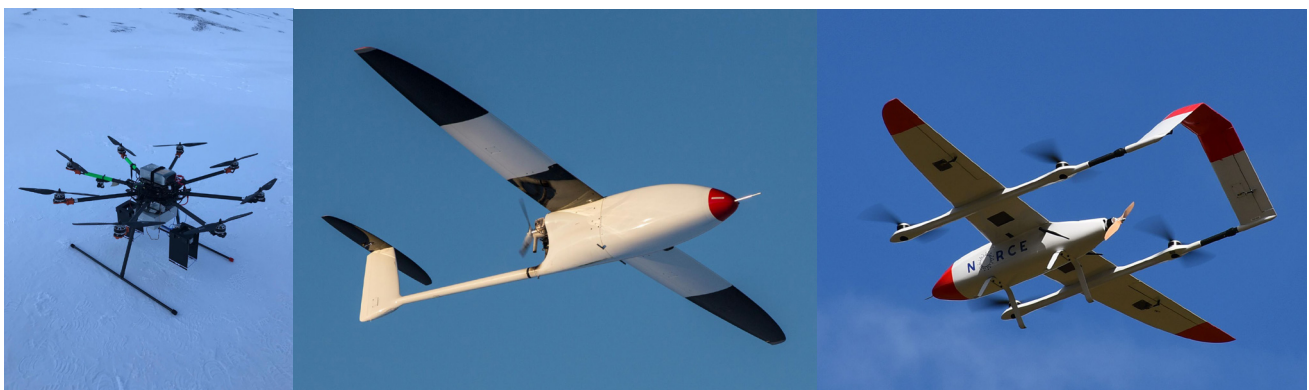
Figure 1: Example of multirotor (left), fixed-wing (middle), and VTOL hybrid (right) used for scientific data collection and part of the SIOS infrastructure (Photos: NORCE).
