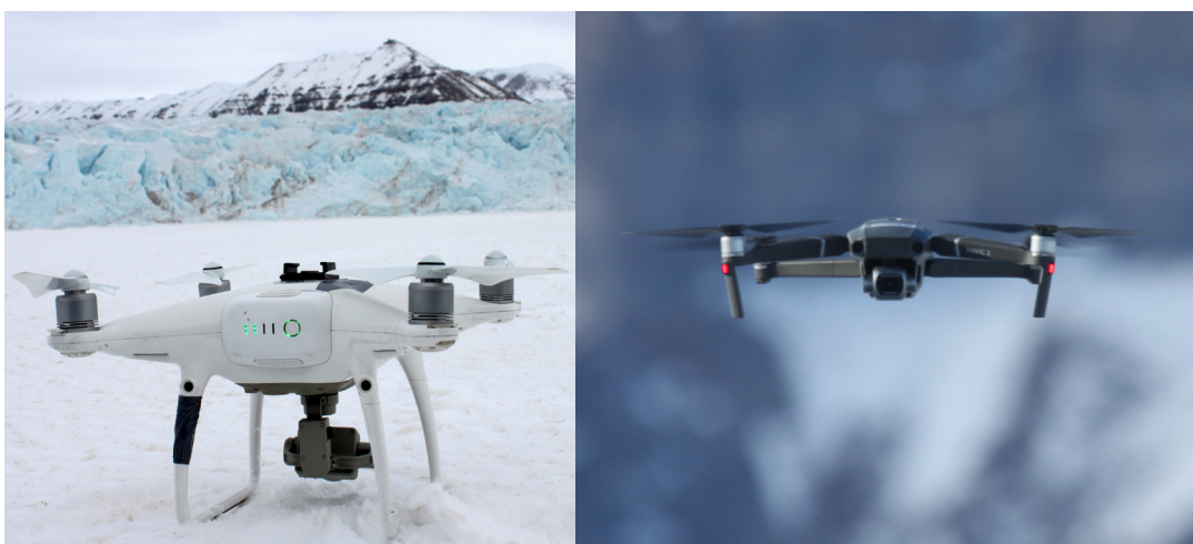
Figure 2: Example of off-the-shelf drones from DJI: Phantom 4 Pro (left) and Mavic 2 Pro (Photos: Richard Hann).
