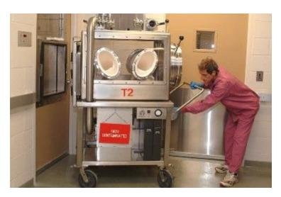
Example of a mobile Class III BSC (Biosafety Cabinet) — suitable for a BSL-4
