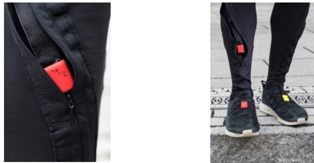
Figure 5: Body Integration of MIMU Motion Capture System
