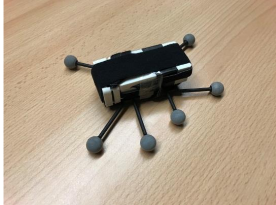
Figure 7: Rigid Body setup of IMU with Infrared Optical Markers for Combined OptiTrack® and IMU Tracking
