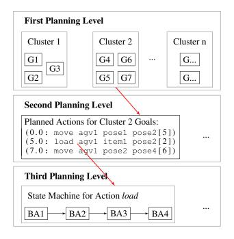
Figure 1: Structure of the Three-Level Planning approach with an example
