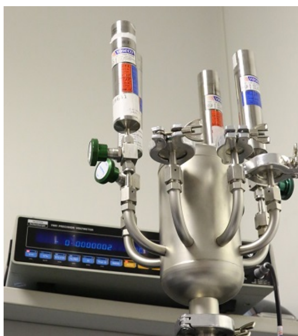
Figure E5.1: Reference leaks externally mounted on a leak detector (photograph courtesy of Vaseco Ltd.)
