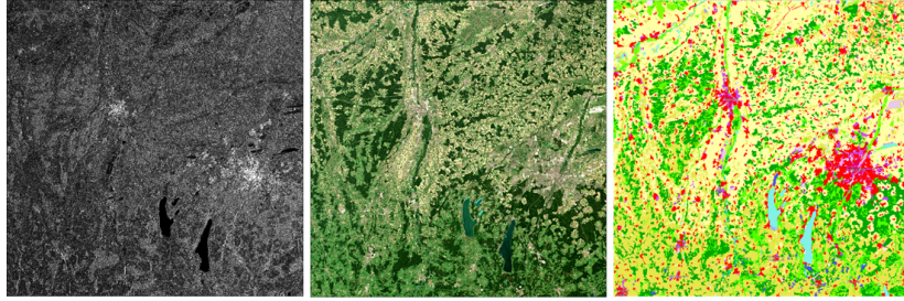
Fig. 6. Munich, Germany as a data fusion example. Left: S-1 image, Middle: S-2 image, Right: CORINE land cover 2018.
