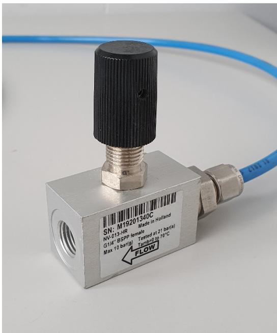
Figure S 2: Picture of the needle valve used (Bronkhorst precision valve, NV-004-HR).
