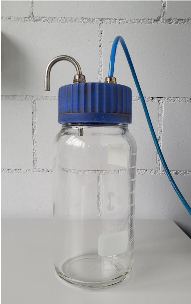
Figure S 1: Picture of an empty sampling glass bottle, including screw cap, waterproof threads, metal tube, and plastic tubing.
