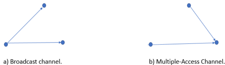
Figure 2. The 3-node relay channel can be viewed as a combination of two channels, a broadcast channel with the source transmitting to the relay and the destination; and a multiple-access channel with source and the relay transmitting to the destination
