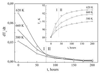
**Figure 4.** Kinetic dependence of the superconducting transition onset temperature  $(T_c, K)$  for the YBa<sub>2</sub>Cu<sub>3</sub>O<sub>7-8</sub> crystals annealed at  $pO_2 = 5 \times 10^5$  Pa and at various temperatures under isothermal conditions.
