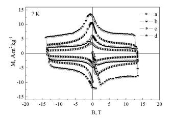
**Figure 2.** Field dependences of the magnetization of the  $YBa_2Cu_3O_{7-\delta}$  single crystal; a, b, c and d after the first, second, third and fourth annealing stages, respectively.
