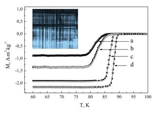
**Figure 1.**  $YBa_2Cu_3O_{7,\delta}$  single crystal magnetization as a function of temperature after thermocycling annealing: a, b, c and d after the first, second, third and fourth annealing stages, respectively. Inset shows crystal surface image in polarized light.
