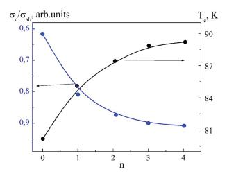
**Figure 3.** Influence of the number of thermocycling annealing processes on the anisotropy of conductivity and the onset temperature of the  $YBa_2Cu_3O_{7-\delta}$  crystal transition to the superconducting state.
