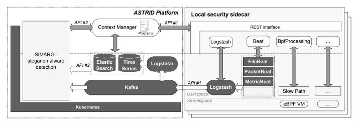
Fig. 1. Software architecture of the ASTRID platform.
