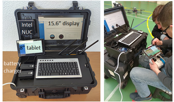
Fig. 1. The Base Station to operate the platform. (Left) Ground Control Unit (including an Intel NUC computer, a 15.6 inch. screen, a keyboard and mouse, a dual-band router and three battery chargers) and a tablet PC showing the GUI. (Right) A human operator using the base station and providing commands to the MAV through the remote controller.
