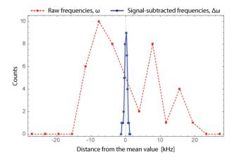
Figure 3 Plot of the distribution of our frequency measurements around their mean value for the raw measurements (dashed red) and the frequencies resulting from the signal subtraction (solid blue). Notice that the subtraction reduces frequency spread by over an order of magnitude, due to common mode noise.
