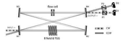
Figure 1 Drawing of the CRDP cavity set-up, showing the cavity mirrors (M1-M4), the flow cell and the coil used to produce the magnetic field, as well as the polarizers P1, 2 used at the output of the cavity. Adjusted on each side of the evacuated cell are 2 anti-reflection coated windows not shown here.
