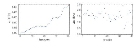
Figure 4: Consecutive measurements of a) the polarization beating frequency observed in one channel (CW propagation, positive magnetic field) b) the beating frequency corresponding to optical rotation, obtained after two signal reversals.
