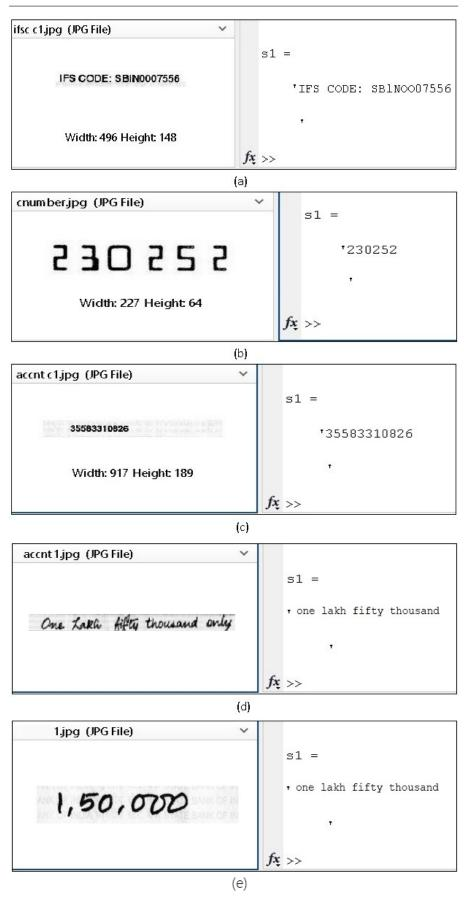
**Fig. 16** Image segments on left hand size and their OCR results (shown as value of s1) for machine printed and handwritten characters on right hand side for (a) IFS code, (b) cheque number, (c) account number, (d) legal amount, and (e) courtesy amount.
