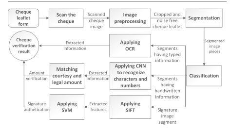
Fig. 5 Block diagram of bank cheque verification process
