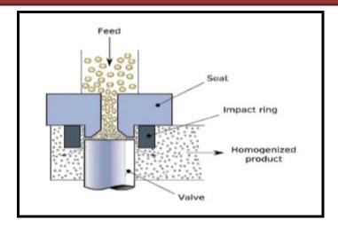
Fig 1:- High pressure homogenization.
