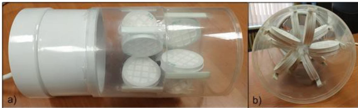
Fig. 5. Photographs of the experimental arrangement used to test the repeatability of the silica aerogel method: the fan, the tube and the thoron samplers can be seen in the picture.
