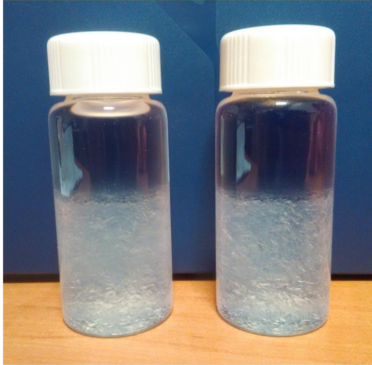
Fig. 3. High performance LS glass vials (20 ml) filled with silica aerogel and Ultima Gold LLT LS cocktail. The photograph is taken after the vials had been placed for 10 min in a ultrasonic bath. When filled with LSC cocktail, the aerogel becomes translucent.
