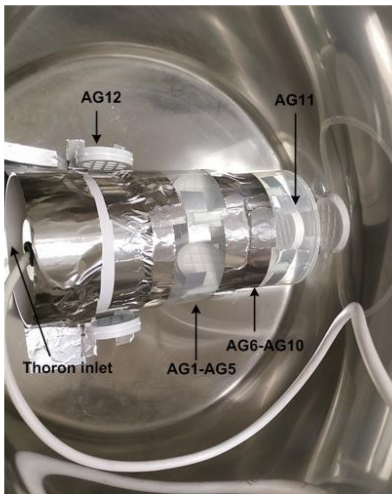
Fig. 6. Photograph of the exposure set-up used to test the repeatability of the silica aerogel method. The fan and the tube with the samplers are placed in a 50 L vessel. Additional samplers are placed in front and near the tube.
