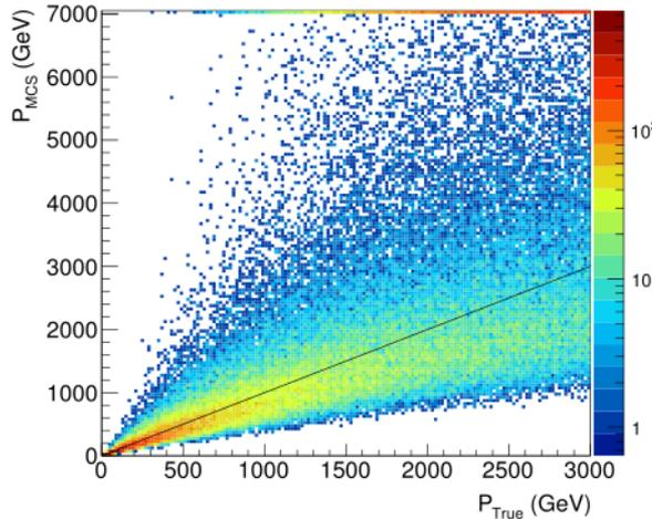
Performance with position resolution of 0.4  $\mu\text{m}$ , in 100 tungsten plates (MC)
