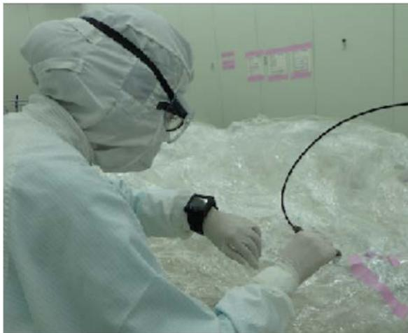
③ He leak test + repairs
