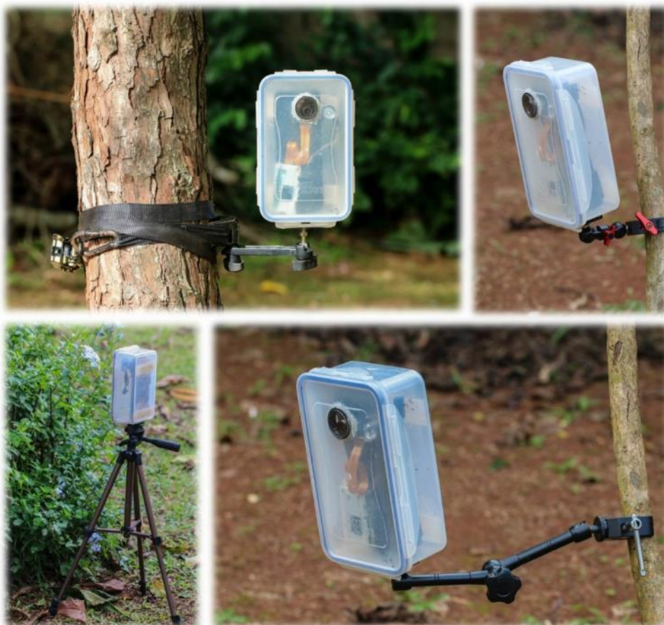
Figure 3. Example of various camera mounts that we successfully tested in the field.
