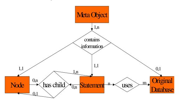
Fig. 5 The relationship between nodes and statements. Each node can have one parent node. A node may have child nodes and statements. Each statement can be linked to an arbitrary number of nodes. A statement is executed by the database it was built for. For nodes as well as statements and the original databases meta information is available.
