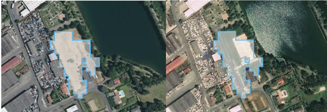
Figure 46. Example showing a change detected as Industrial (overlaid on an orthophoto for 2016 on the left and 2019 on the right) by the CDS and considered as industrial by the reference.
