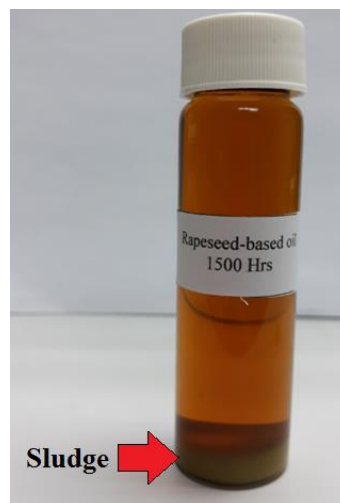
Figure 9. Formation of sludge in the rapeseed oil after 1500 h of aging
