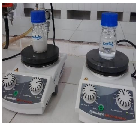
Fig.1: Preparation of PLA/Ag using Nanosilver powder
