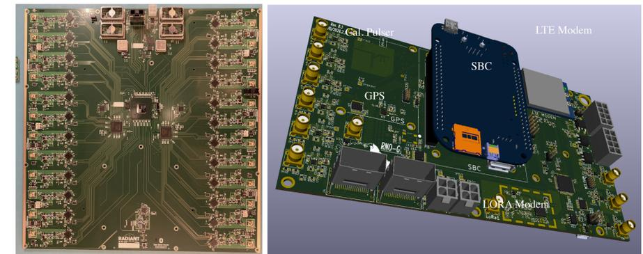
Fig. 6: Left: 24 channel RADIANT digitizer board. Right: Controller board with SBC in place.
