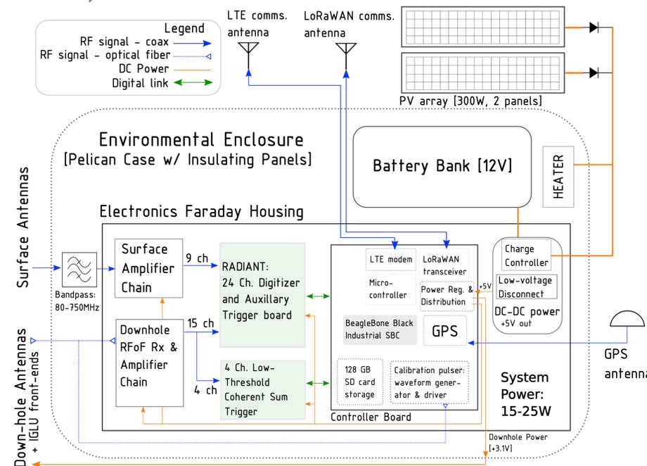
Fig. 4: Surface stations electronics diagram, including power, comms., calibration pulser, and DAQ.
