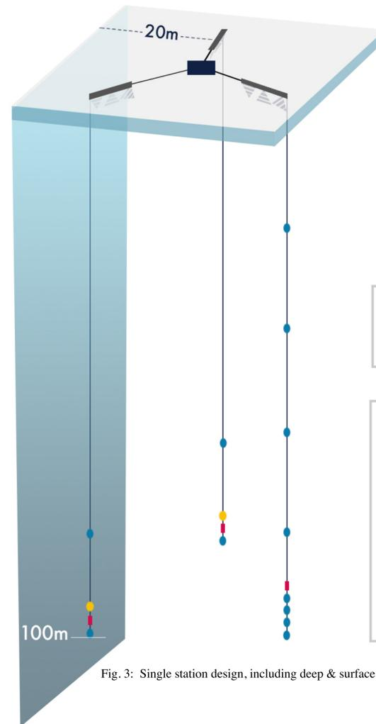
Fig. 3: Single station design, including deep & surface antennas and the DAQ box.
