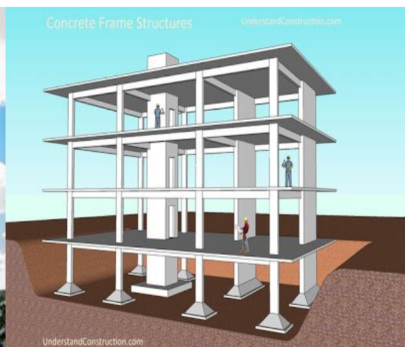
Fig.2:-RCC framed structure
