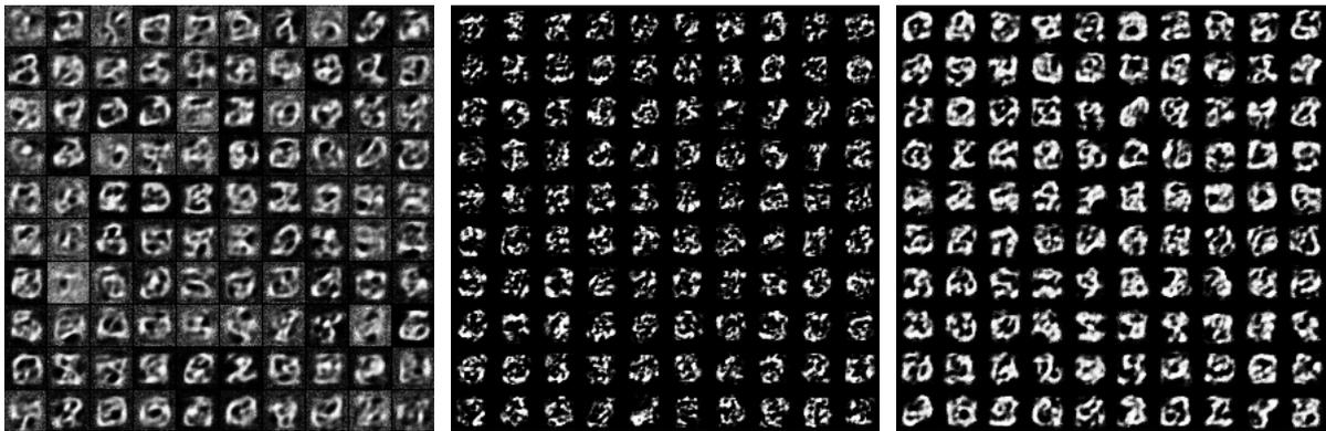
Figure 5.6.8: Input reconstructions of the single activations in a third layer respectively for a DBN (left), SA (center) and SdA (right), trained on MNIST-50.
