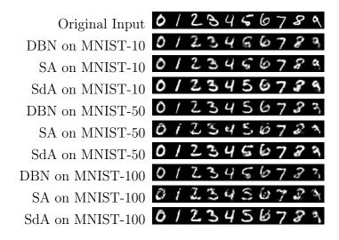
Figure 5.6.10: Reconstruction of the input, by each of the three architectures, starting from the third layer internal representations of the first-10-digits in the test sets for MNIST-10, MNIST-50 and MNIST-100.
