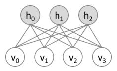
Figure 2.4.1: Graph of a Restricted Boltzmann Machine.  $v_j$  is a visible unit and  $h_j$  is a hidden unit. In an RBM, connections are exclusively drawn between visible units and hidden units.
