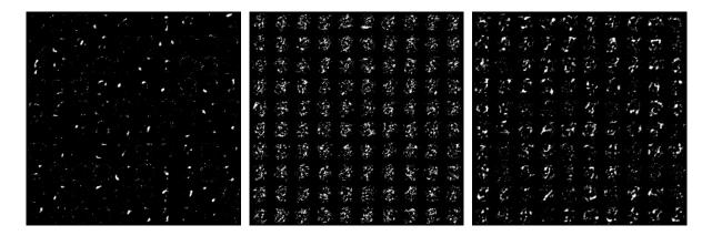
Figure 5.6.4: 100 random out of 400 input reconstructions of the single activations in a second layer respectively for a DBN (left), SA (center) and SdA (right), trained on MNIST-10.
