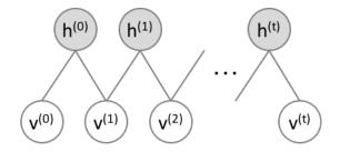
Figure 2.4.2: Steps of Gibbs sampling in a Restricted Boltzmann Machine. v are visible units and h are hidden units. Each step is performed from a visible unit to hidden unit, or vice versa.
