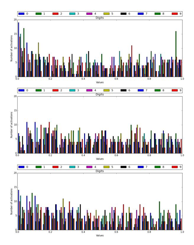
Figure 5.4.6: Histograms of third layer internal representations of the Mean-Digits respectively for a DBN (top), SA (middle) and SdA (bottom), trained on MNIST-50. The y-axis shows the number of activations, the x-axis has 20 bins for values in range [0, 1]. Each color represents a different digit.
