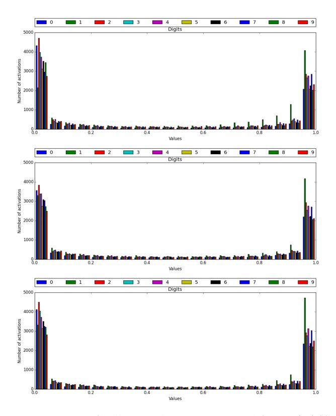
Figure 5.4.2: Histograms of third layer internal representations respectively for a DBN (top), SA (middle) and SdA (bottom), trained on MNIST-10. The y-axis shows the number of activations, the x-axis has 20 bins for values in range [0, 1]. Each color represents a different digit.
