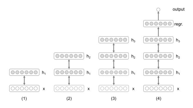
Figure 3.1.1: Layer-wise training of a Deep Belief Network, composed by stacked RBMs. From the bottom,  $\boldsymbol{x}$  is the input and  $\boldsymbol{h}_{\boldsymbol{k}}$  are hidden layers. (1) The first layer is trained. (2) The second layer is trained using the first hidden layer as visible units. (3) The third layer is trained using the second hidden layer as visible units. (4) A regression layer is added and the resultant DBN is ready for the fine-tuning.
