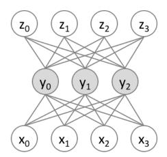
Figure 2.2.1: Graph of an Autoencoder. From bottom to top, respectively, the input layer (white), the hidden layer (gray) and the output layer (white).  $x_k$  is an input unit,  $y_j$  is a hidden unit and  $z_k$  is an output unit. Connections are exclusively drawn between different layers.
