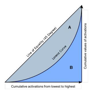
Figure 4.3.1: A Lorenz curve for an internal representation. A is the area between the equality 45-degree line and the Lorenz curve generated by the sequence; B is the area under the Lorenz curve. The Gini coefficient is proportional to the ratio of the areas A/B.
