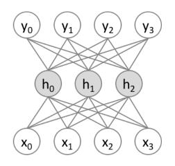
Figure 2.1.1: Graph of a multi-layer perceptron with one hidden layer. From bottom to top, respectively, the input layer (white), the hidden layer (gray) and the output layer (white).  $x_k$  is an input unit,  $h_j$  is a hidden unit and  $y_k$  is an output unit. Connections are exclusively drawn between different layers.
