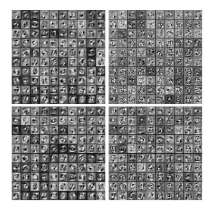
Figure 5.5.3: Third layer original sorted filters. The top row contains respectively a DBN filter set (left) sorted to match a SA filter set (right). The bottom row contains respectively the same DBN filter set (left) sorted to match a SdA filter set (right). All architectures are trained on MNIST-10.
