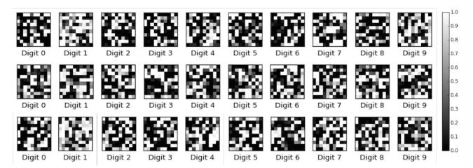
Figure 5.4.1: Internal representations in the third layer of the first 10 digits of the MNIST-100 test set, respectively for a DBN (top), a SA (middle) and a SdA (bottom). These internal representations are obtained by feeding the original digits to the network.
