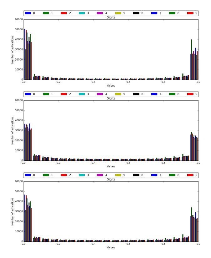
Figure 5.4.4: Histograms of third layer internal representations respectively for a DBN (top), SA (middle) and SdA (bottom), trained on MNIST-100. The y-axis shows the number of activations, the x-axis has 20 bins for values in range [0, 1]. Each color represents a different digit.
