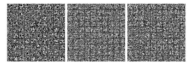
Figure 5.6.1: 100 random out of 900 input reconstructions of the single activations in a first layer respectively for a DBN (left), SA (center) and SdA (right), trained on MNIST-10.
