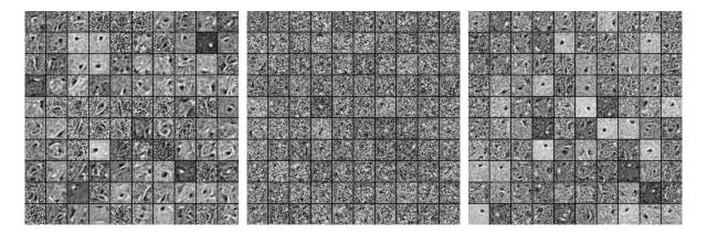
Figure 5.3.2: 100 random out of 900 first layer filters respectively for a DBN (left), SA (center) and SdA (right), trained on MNIST-50.
