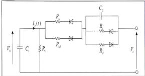
Figure 1. Equivalent circuit of Thevenin model
