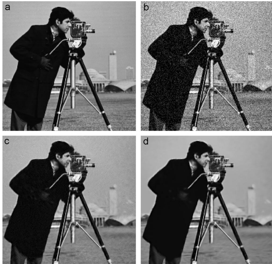
Figure 6: PCA in image denoising task [22]. (a) Original image Cameraman; (b) noisy image (c) denoised image after the first stage of the proposed PCA-based method and (d) denoised image after the second stage.
