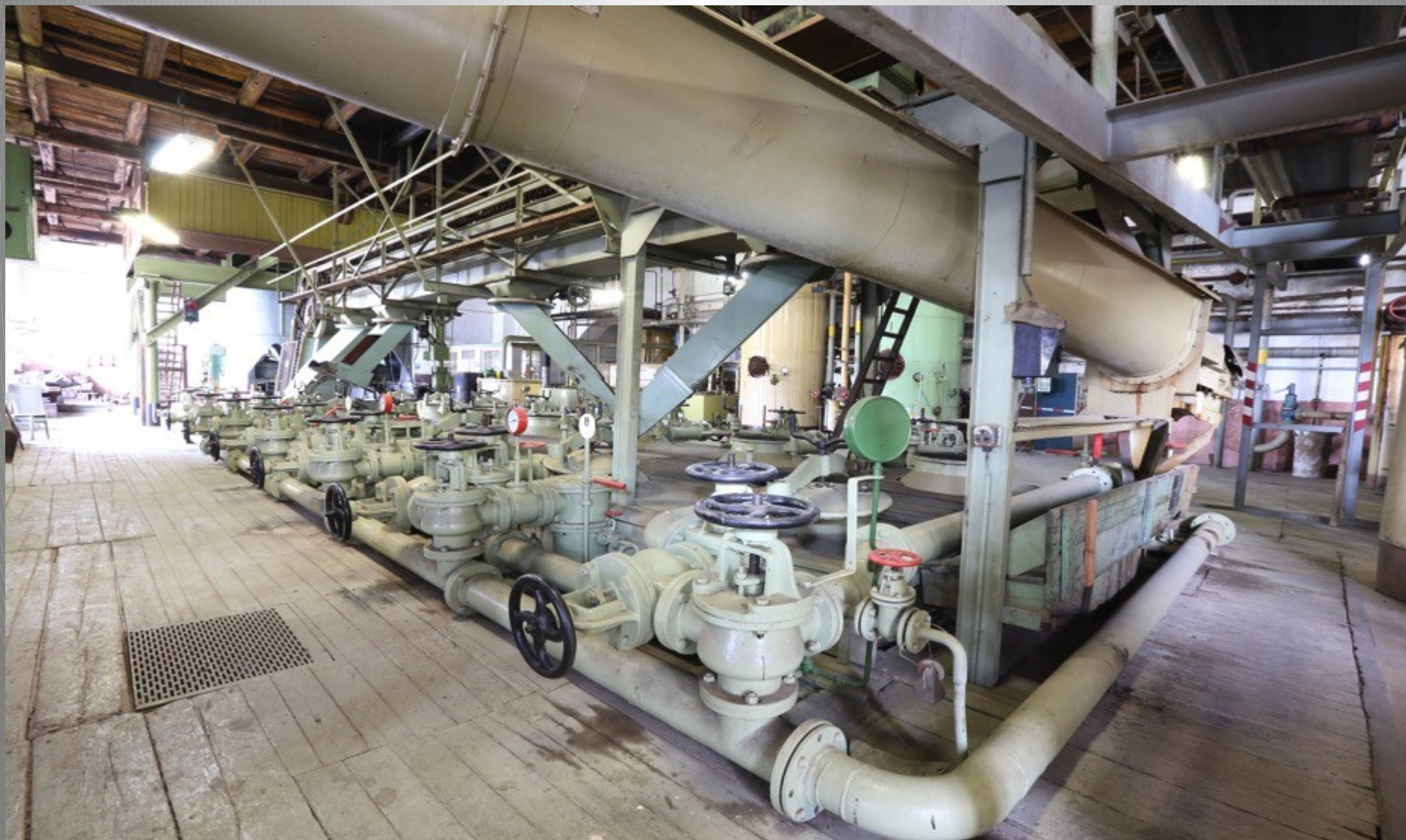
Diffuser battery dating back 1906, Every eight minutes, a cell was loadet with fresh cossetes
