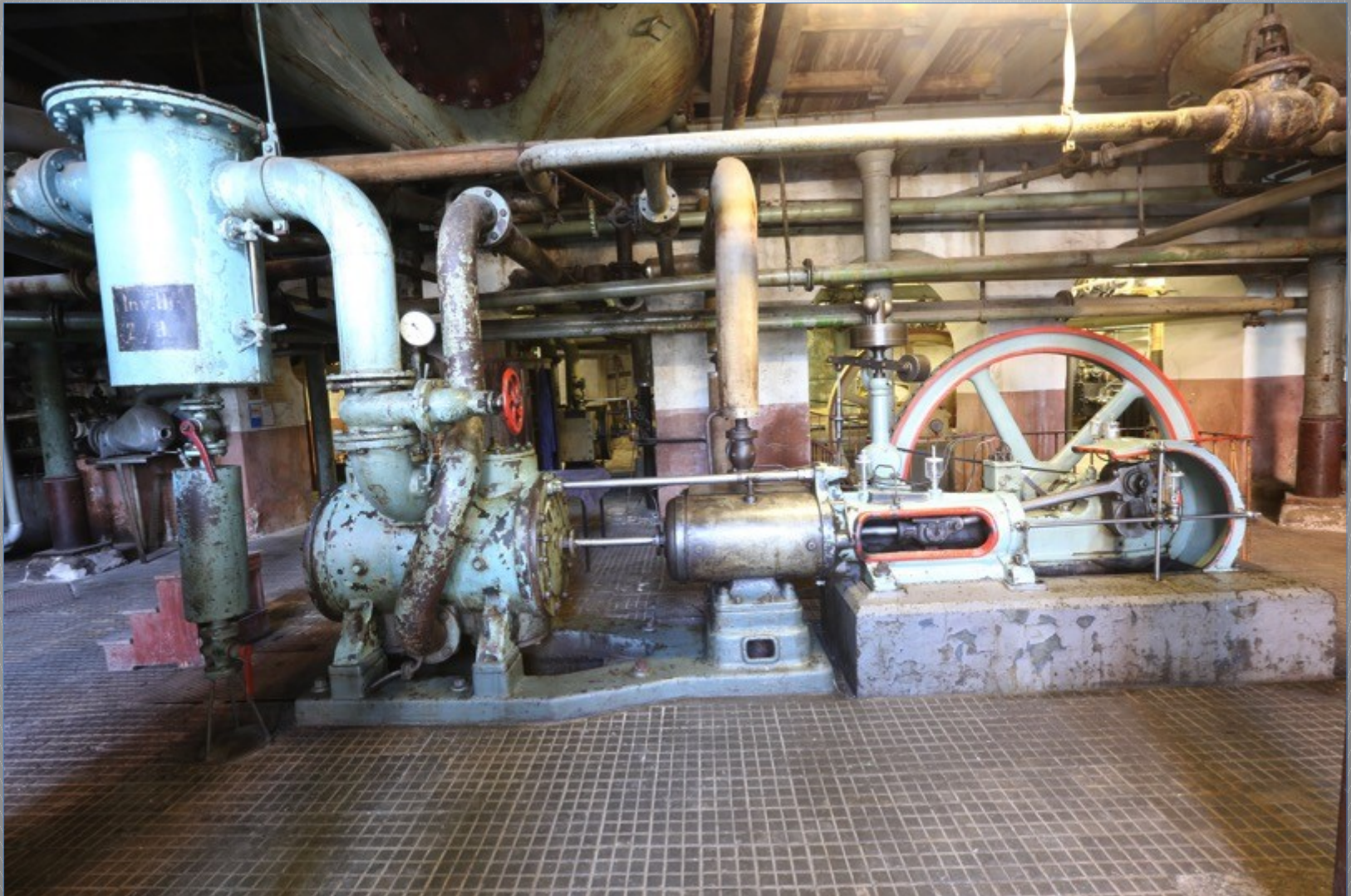
Horizontal one-cylinder steam engine driving the vacuum pump of the condenser of the evaporator station, built in 1925 bei Braunschweigsche Maschinenbauanstalt
