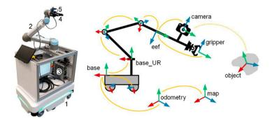
Fig. 4. Use case example: adaptive mobile manipulator including frames and kinematic structure.
