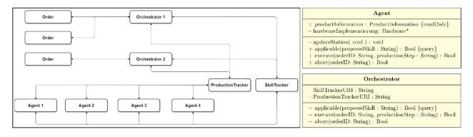
Fig. 1. Communication architecture of the UAS TW Digital Factory.
