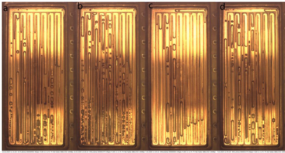
Figure 3: Flow images belong to E:H = 1:4 and E:H = 4:1 at vertical condition ( 90^\circ ).
