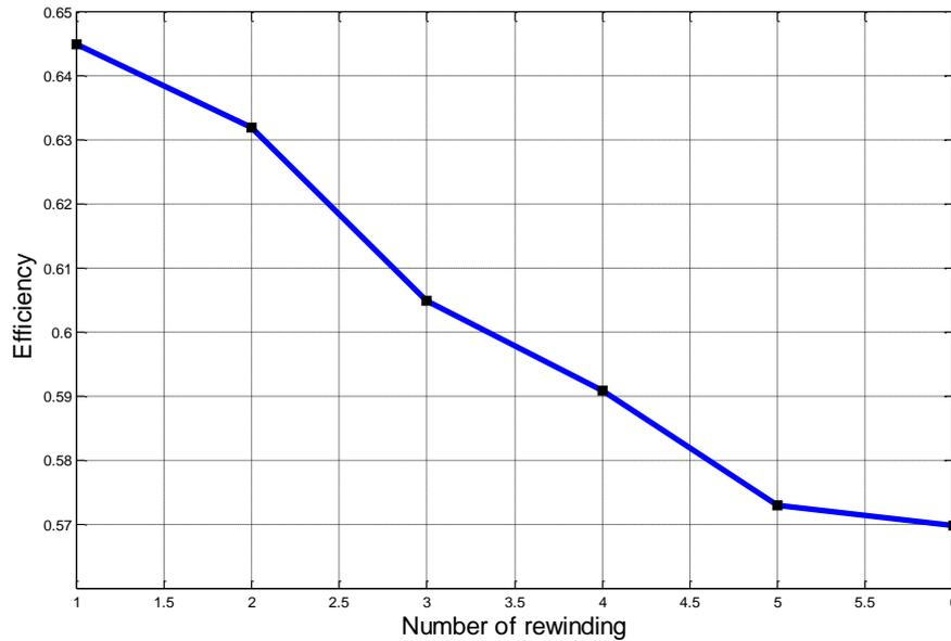
Figure 1. Efficiency dependence on the number of rewinds
