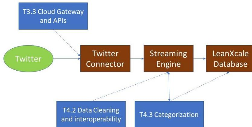
**FIGURE 10 - DATASET CATEGORIZATION PIPELINE INTEGRATION**
