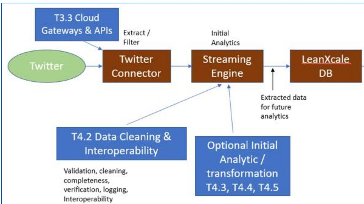
**FIGURE 4 - THE STREAMING DATA PATH**
