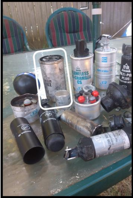
Fig. S9. Deployed hexachloroethane grenade 9: 19 July 2020, unknown location, detonated, not observed deployed, recovered. Note the coloration and dimensions of the can (e.g., the rim shape and size) are distinct from the standard HC Military Style Maximum smoke whether unexploded (Fig. S1) or exploded (Fig. S7), suggesting perhaps a different run of product or a partial detonation. (14)
