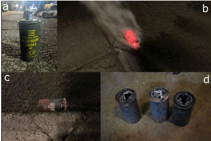
Figure 3. Hexachloroethane (HC) / Zinc Oxide canisters: (a) Unexploded ordnance clearly marked as “Military Style Maximum Smoke HC” from “Defense Technology”; (b) HC ordnance off gassing Zinc Chloride mid-deployment; (c) Same canister from (b) after reaction stopped, showing charred remains of the label that matches the canister in (a); and (d) three exploded HC canisters, including the one from (b) and (c) in the middle. Photos (a) and (d) from the author, (b) and (c) from Sarah Riddle and used with permission.
