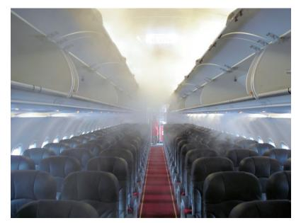
Condensation on AirAsia flight AK6303 with A320 from Langkawi (LGK) to Kuala Lumpur (KUL). Departure in tropical rainforest climate ("PlaneHunter", <a href="http://bit.ly/2oUJYKP">http://bit.ly/2oUJYKP</a>)
