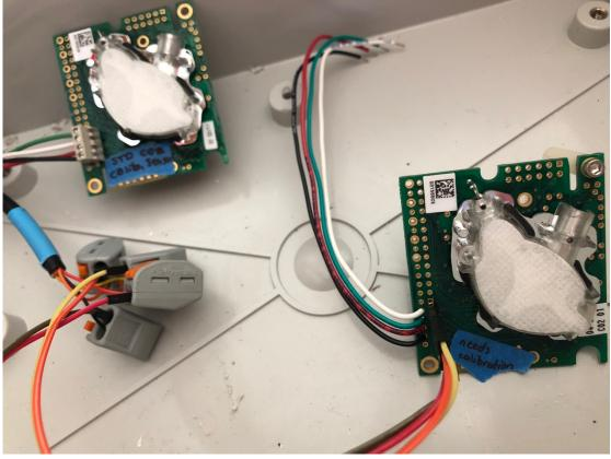
5. If the calibration sensor has not already been set up, (with terminal block in the top right corner) in descending order: Black, Red, White, Green.
