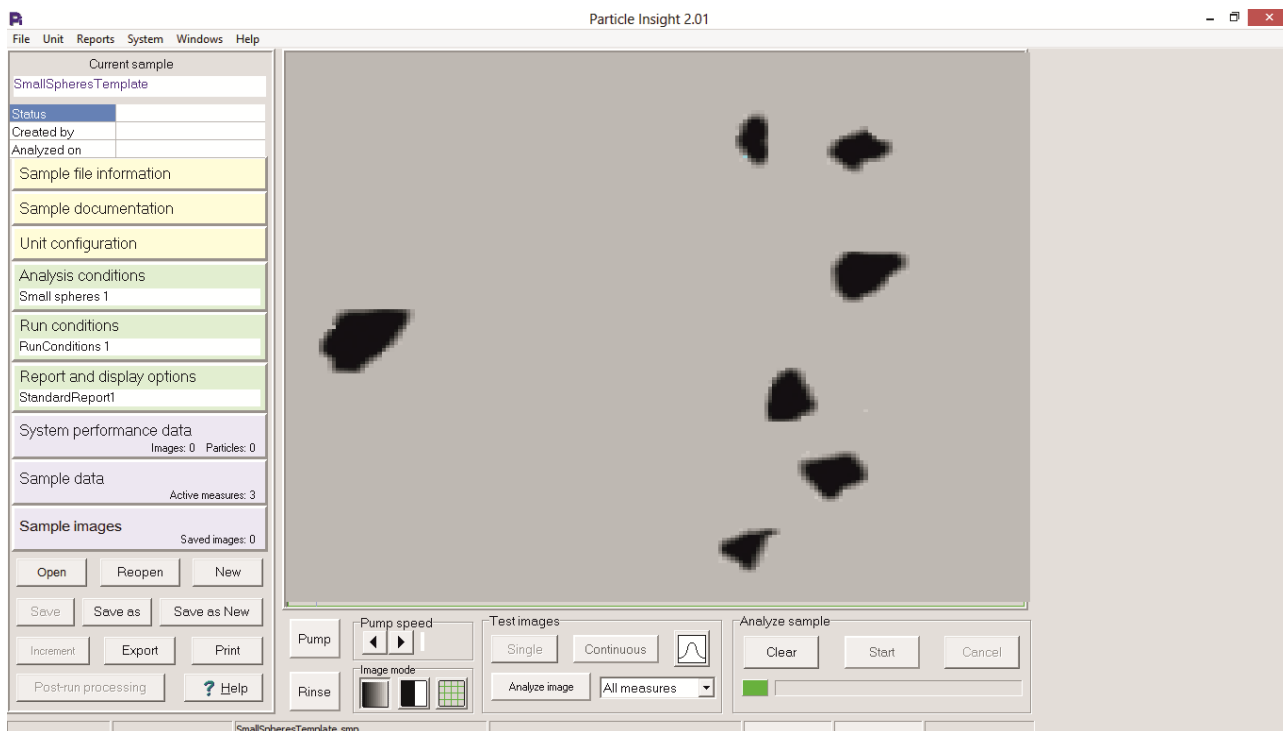
Fig. 4. Screenshot from the program interface used in DIA instrument called Particle Insight 2.01 (Micromeritics®) [32]
