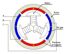
Figure 1. BDCM simple cross section.
