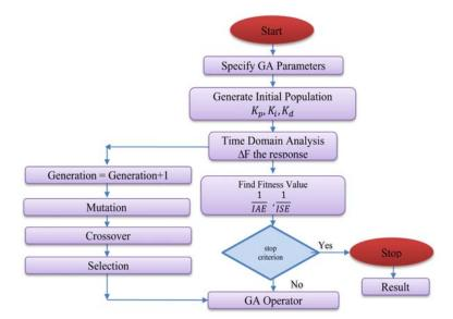
Figure 7. Proposed genetic algorithm process design flowchart. Area of error for the system response
