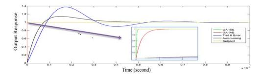
Figure 9. Step responses for PID/GA, trial & error and conational PID controllers
