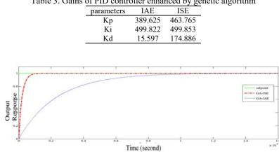
Table 3. Gains of PID controller enhanced by genetic algorithm
