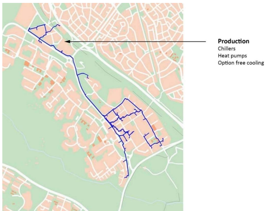
Figure 22: The second largest Stockholm system, the Kista system, designed for 50 MW [17]
