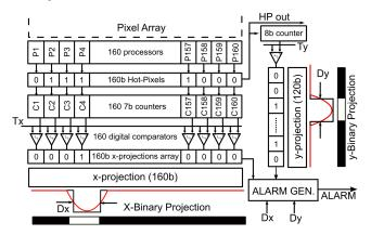
Fig. 5: Schematic of the circuit for alert generation relying on the HP XY projections.
