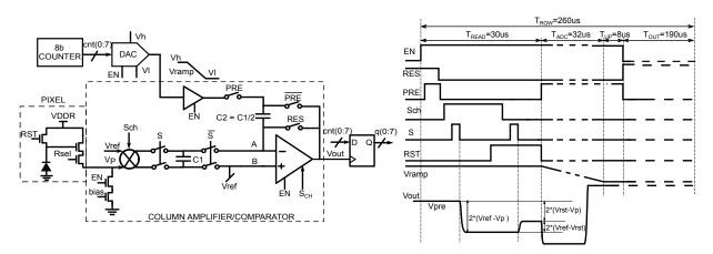
Fig. 4: Schematic of the single-slope ADC where, after the pixel readout, the chopper amplifier is converted into a comparator as part of the ADC. On the right, the timing diagram of the pixel readout ( $T_{READ}$ ), ADC ( $T_{ADC}$ ), threshold update ( $T_{UP}$ ) and data dispatching ( $T_{OUT}$ ) is shown for a sensor frame rate of 8fps.
