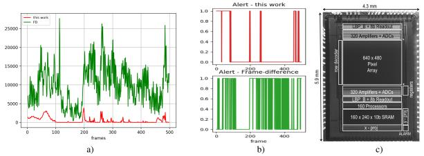
Fig. 8: Hot-pixel activity of this sensor compared to the FD counterpart. The comparison refers to the video of Fig. 7. From frame 90 to 500 the boat is outside the scene and no events should be detected; b) activity of the alert signal generated by the two approaches; c) microphotograph of the VGA sensor measuring  $25.4 \text{ mm}^2$ .
