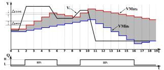
Fig. 1: Operating principle of the sensor embedded DT-DBS. In this case, the pixel voltage  $V_i$  changes abruptly while  $V_{Max_i}$  and  $V_{Min_i}$  approach  $V_i$  at two different speeds, according to (2) and (3).
