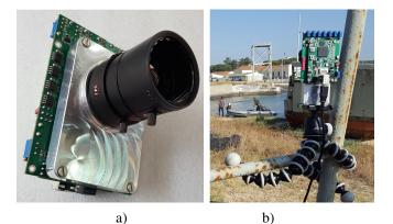
Fig. 9: Sensor prototype: a) the vision sensor is driven by a FPGA and interfaced with a PC through which it is possible to change the algorithm parameters and grab grayscale videos with related motion bitmap, projection vectors and alert; b) test setup used in outdoor scenario.
