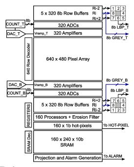
Fig. 3: Block diagram of the VGA vision sensor architecture.
