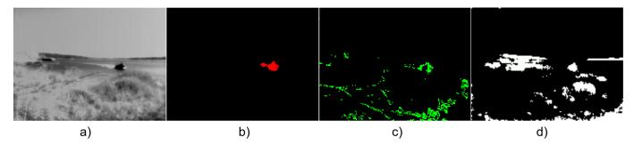
Fig. 7: a) VGA grayscale image captured with the fabricated chip; b) motion bitmap delivered by the proposed vision sensor in a real outdoor scenario; c) motion bitmap generated simulating FD algorithm applied on the video in a) and scaled to QQVGA resolution in order to be normalized with this sensor. d) Hot-pixel bitmap generated by traditional Background Subtraction (BS). The number of hot-pixels generated by FD and BS is much larger than that of DT-DBS.
