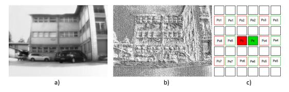
Fig. 6: a) Gray-scale image captured by the fabricated sensor with b) its LBP coding delivered by the sensor. c) 5x5 pixel kernel used to compute LBPs. Pixel Pe refers to the neighbouring pixels Pe1-Pe8 and is computed with the Bottom-Side block, while Po refers to Po1-Po8 and is executed by the Top-Side block of the VGA array.
