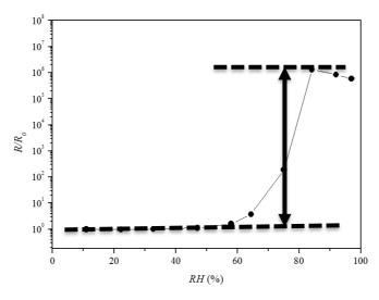
Fig. 4. Huge jump of electrical resistance of a water sensor at the percolation point RH=80% [12], note the logarithmic scale.
