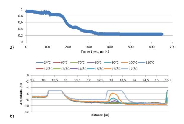
Fig. 7. Sigmoidal trend of light transmission through a polymer optical fibre a) when a target temperature of 135°C is reached, here after 180 seconds. The light transmission that has started at a plateau of almost 1 (100%) and falls down to a steady value of approximately 20%. The plot in time domain reflectometry is given by b), here the sensor starts at 10,5 meters and the defect is applied at 13 meters.
