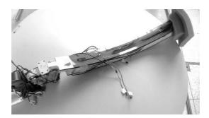
Fig. 2. Slat Track from Airbus A 320 with installed crack propagation of Vishay, partially overpainted.
