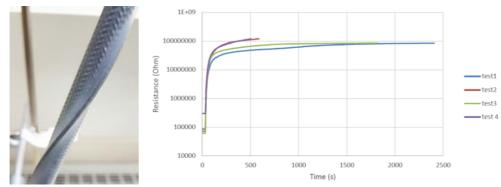
Fig. 5: Sensor wrapped around a hydraulic tube and sensor response recorded when exposed to tiny amounts of hydraulic liquids.
