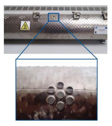
Fig. 6. Demonstrator for the detection of bleed air leakage. Above the pre-set "escape holes" for hot air, a robust polymer optical fibre is installed undergoing glass transition at the target temperature, easily detectable by state-of-the-art optical time domain reflectometry (TDR).
