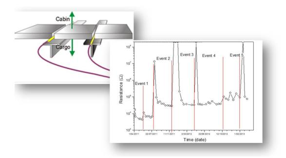
Fig. 8 Wire sensor for detecting "wetness events" in floor structures of a Boeing 737-530.
