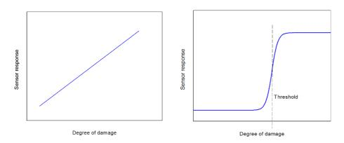
Fig. 1: Principal response of a quasi-linear and a highly non-linear sensing material [1].
