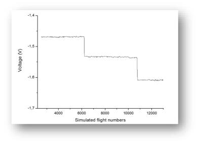
Fig. 3. Readings from crack propagation gauges, the distances between the "steps" represent 0,25 mm.
