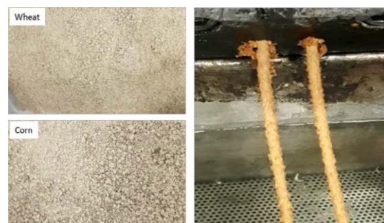
Figure 1: Wheat and corn milled and ready for compounding (left). Detailed of extruded material reinforced with fibers (right)
