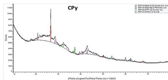
**Figure 1:** Example of XRD diffractogram (CPy sample)
