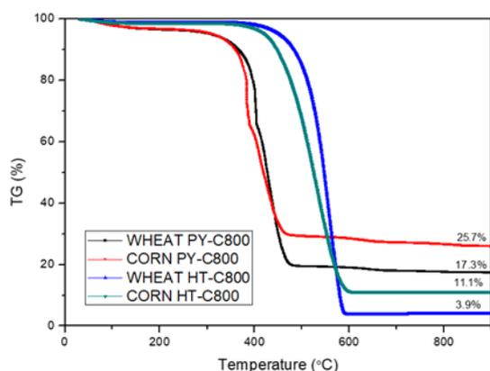
**Figure 3:** TGA profiles of AC samples
